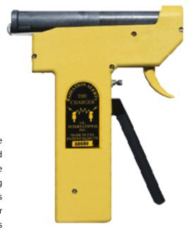
(shown with pencil-type dosimeter in position for charging)
