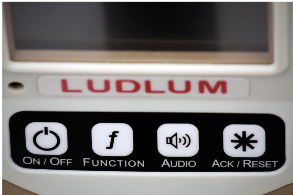
The instrument is equipped with a four-button control pad, as shown above. All controls for the instrument are performed via these four control buttons. Each labeled button has set operation(s) it performs.
