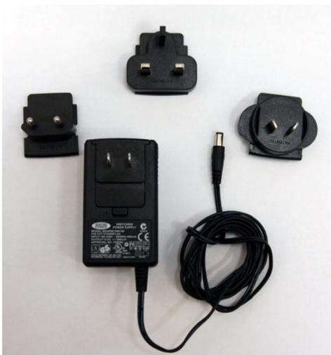
The power charger input accommodates 108-240 V at between 50/60 Hz. The output is 15.0 V at 1600 mA. To ensure proper charging, do not use chargers with other specifications than those listed above. Charging circuitry to monitor battery levels and protect the NiMH batteries from over-charging is all built into the Ludlum instrument.
