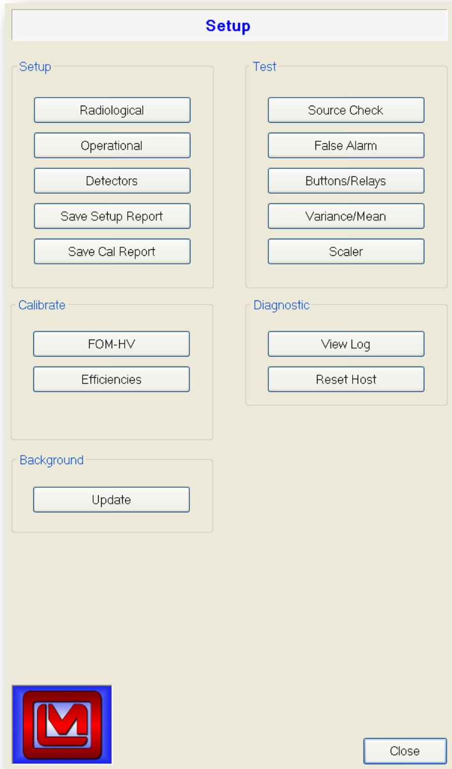
Radiological – Sets up the counting mode and its parameters, isotopic mix, occupancy mode, and units of measurement.
