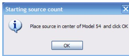
The Gamma Personnel Portal will begin taking source counts at each high-voltage step until completed. Once the current detector is complete, the process will begin for any remaining detectors.
