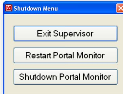
**Exit Supervisor** – Closes the Supervisor application and provides access to the Windows 7 Embedded environment. This is necessary for performing software updates, configuring windows settings, such as printing or networking, or to provide access to the data files. A confirmation window will be displayed before the Supervisor application is closed.
