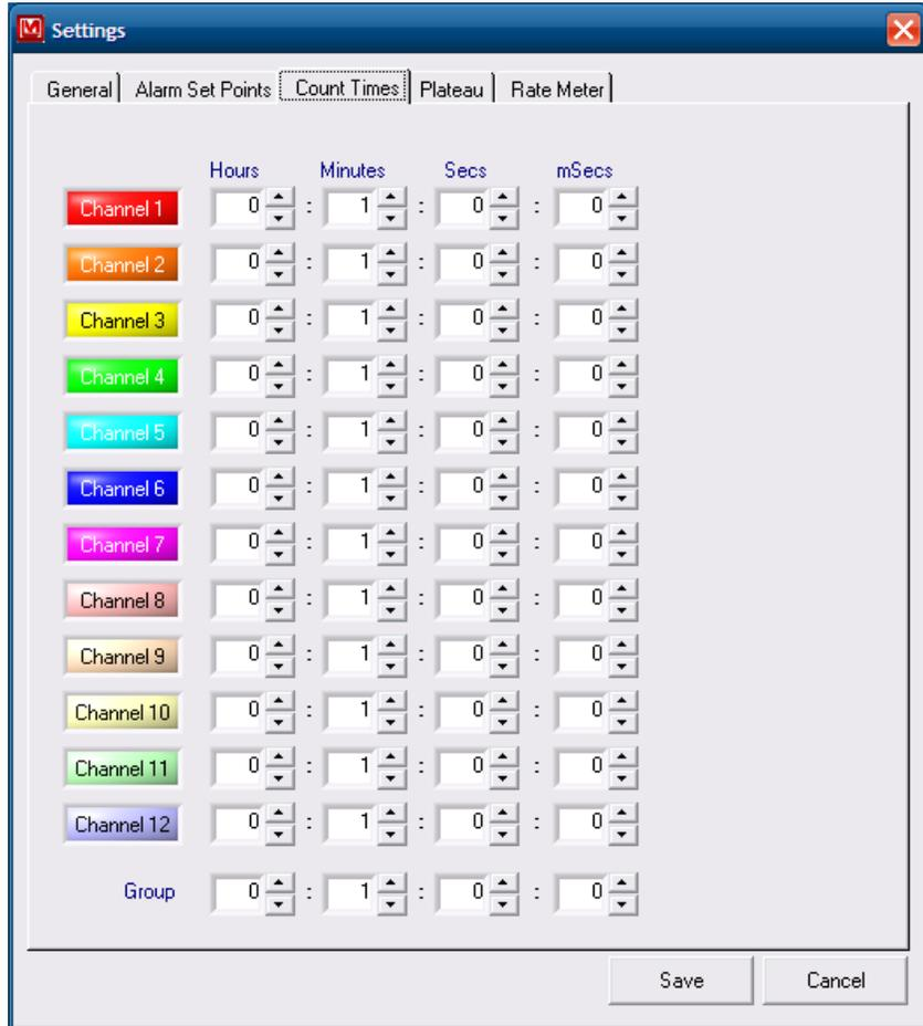
The values here determine the default counts times for each channel. These are just default values and can be changed at any time from the main screen.
