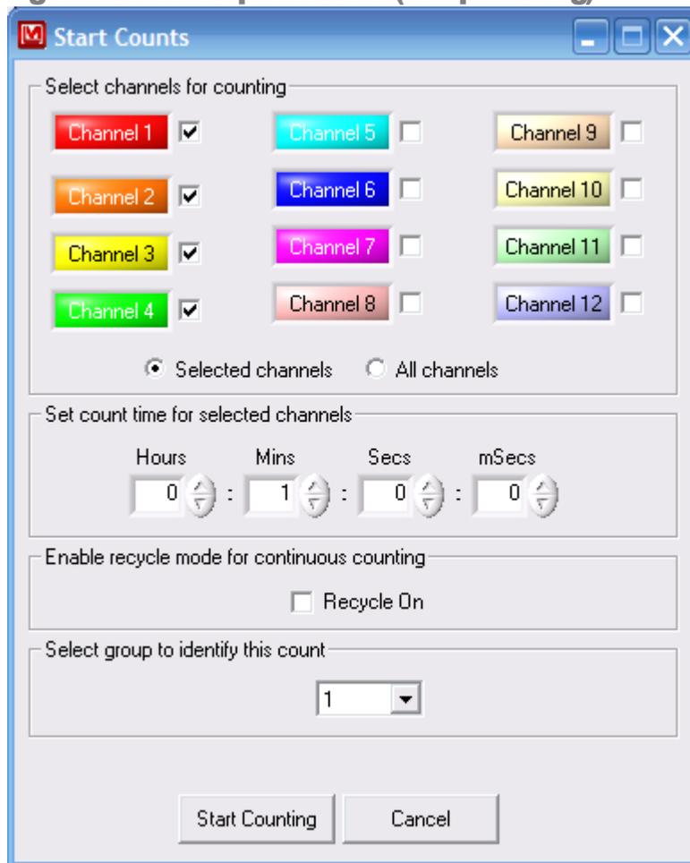
To start counting on a group of channels, click on the “Start” button. From this screen the user can start all channels counting simultaneously or individually select a group of channels. To select an individual channel make sure the “Selected channels” radio button is selected, and then click on either the check box or channel indicator.
