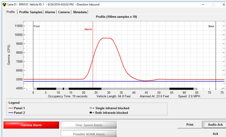
The Alarm window is automatically displayed and an alarm report is printed when a gamma alarm or over-speed alarm occurs. The alarm window is grouped into five tabs, each representing a different aspect of the alarm. The bottom of the alarm popup displays the gamma alarm status, over-speed alarm status, and the direction, date, and time of the occupancy. A Print button allows
