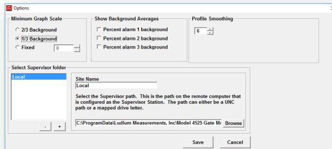
**Minimum Graph Scale:** Specifies the minimum graph scale for the Y-Axis on the profile graphs.
