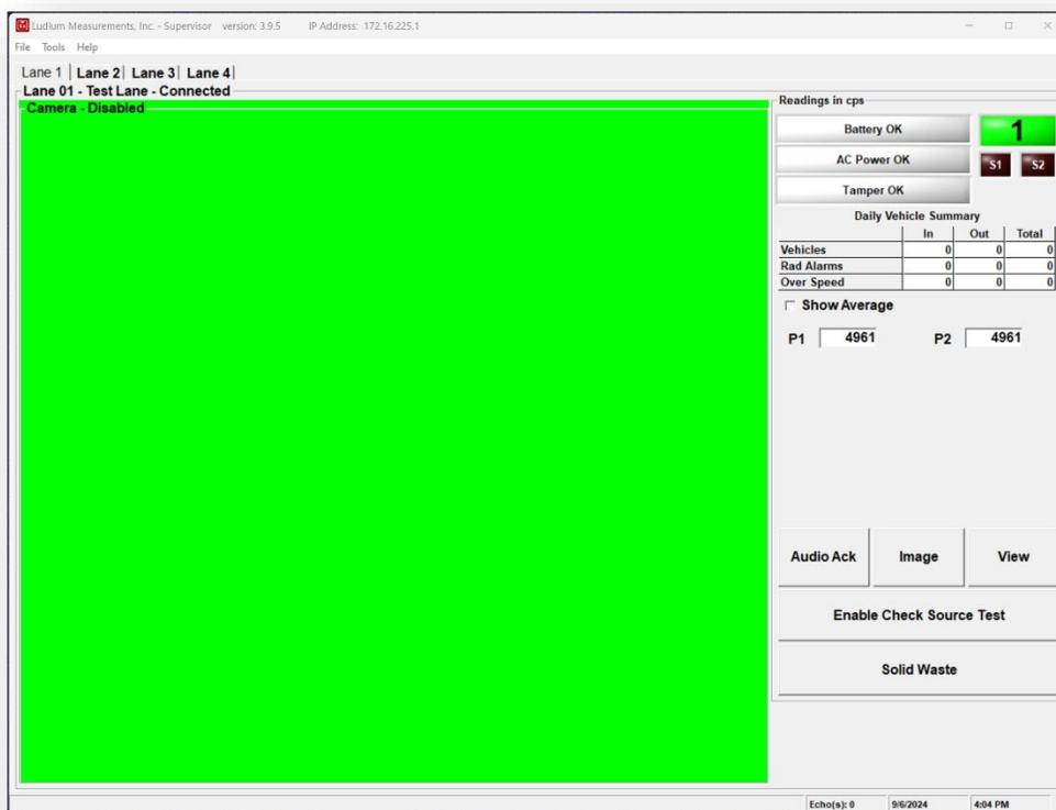
The main screen displays four tabs with each tab displaying the data for one lane. Each tab displays a camera image, battery and AC power status, infrared sensor indicators, and vehicle counts including number of radiation alarms and over-speed alarms, and the current background readings for each panel. There
