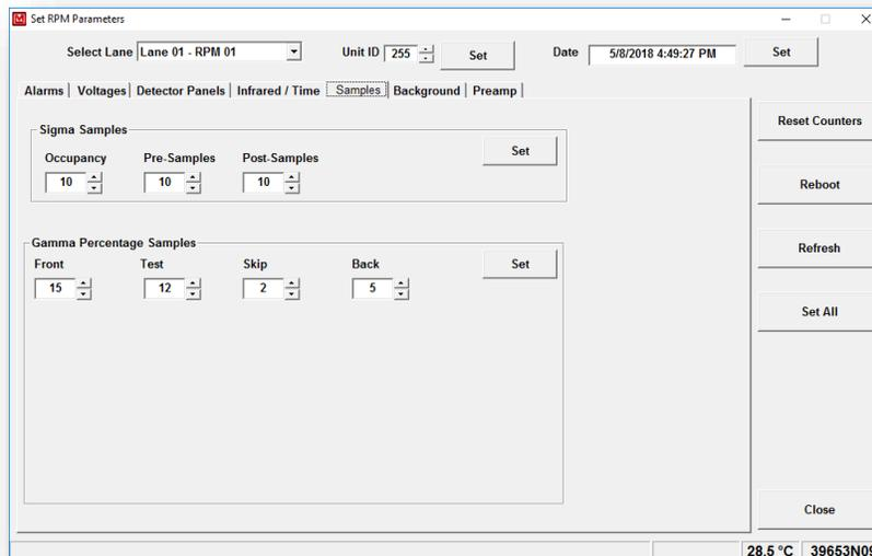
**Occupancy Samples:** Sets the number of 100-millisecond samples that must occur before checking for an alarm. The RPM should be rebooted after changing this parameter.
