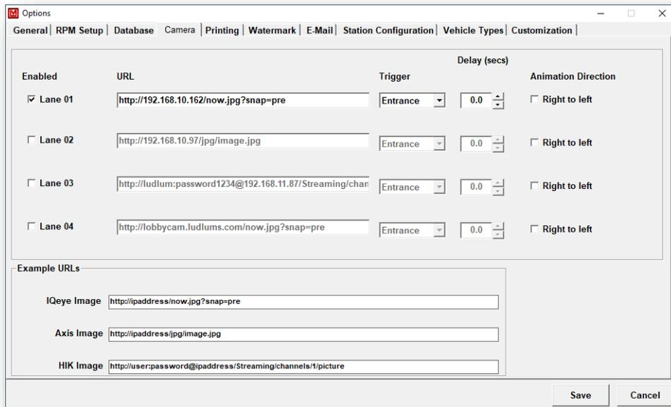
The Camera tab is used to configure an Ethernet camera to be used to capture an image during the occupancy and to display on the main screen. For each camera, a URL is specified that is used to retrieve an image from the camera. The main screen will update approximately every 1 second with a new image. When a vehicle breaks an infrared beam, an image will be captured and will be saved in the event of an alarm. It is also possible to save an image for every occupancy.
