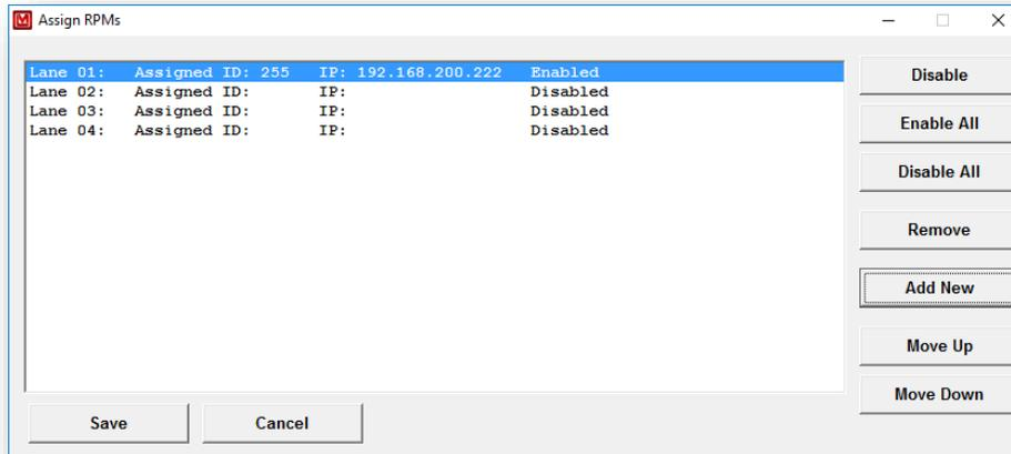
To assign an RPM to a lane, select a lane and click on the Add New button. A list of all unassigned RPMs that were found in the Search screen will be displayed. Highlight an RPM and click on the OK button.
