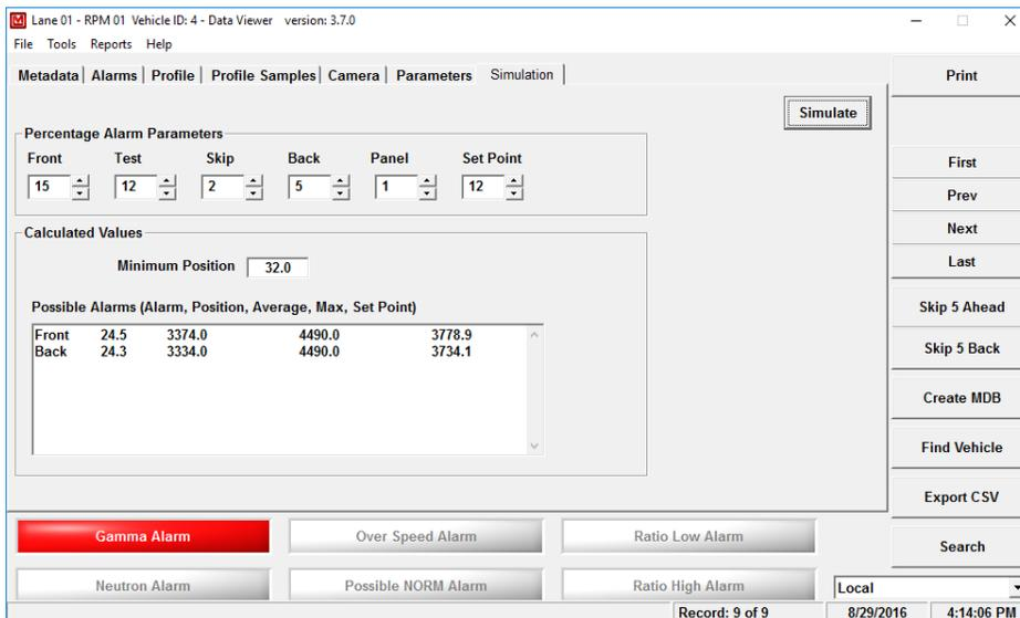
The Simulation tab can be used to modify the percentage alarm parameters and retest the vehicle for a percent alarm. Adjust the samples as desired, and click the Simulate button. The Minimum position of the alarm and the locations of possible alarms are calculated based on the current records' profile data.
