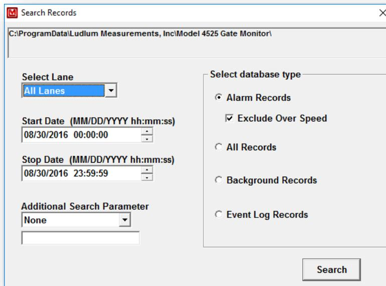
To search the databases, click the Search button on the main screen. After selecting the options to configure the search parameters, click the Search button. The current database path is shown at the top of the window.
