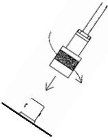
Connect one end of the cable provided to the detector by firmly pushing the connector together while twisting clockwise  $\frac{1}{4}$  turn until latched. Repeat the process in the same manner with the other end of the cable and the instrument.
