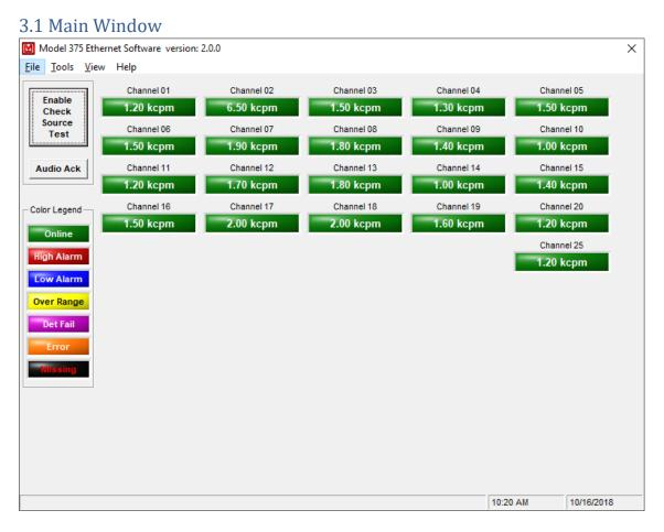
The main window displays reading boxes for all enabled Model 375s along with their status, units, and caption. Left-clicking on the channel will open a web browser to the camera if enabled. Right-clicking on the channel name will display the last image and alarm information that has occurred since the program was running. Holding the mouse over the channel name will display a tool tip with the user-defined comment.
