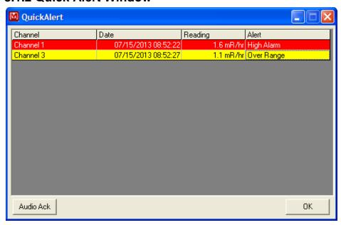
When any type of failure or alarm occurs, this window is displayed showing the channel, date, reading, and type of event. This data is available until the window is closed. Click the **Audio Ack** button to silence the audio.
