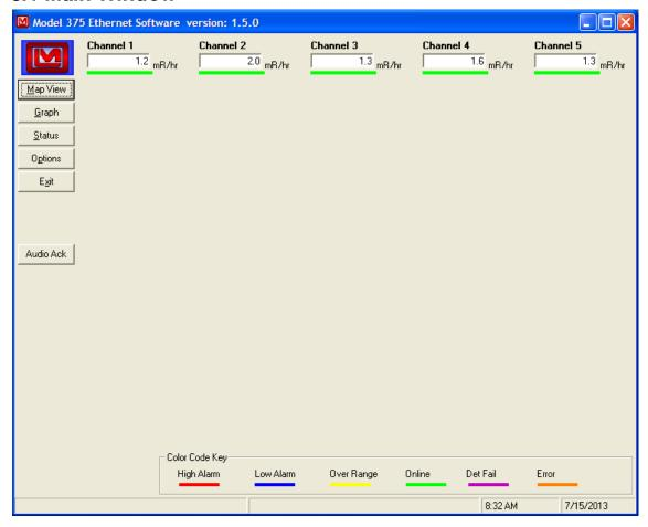
The main window displays reading boxes for all enabled Model 375s along with their status, units, and caption. Clicking on the channel name will display the last image and alarm information that has occurred since the program was running. Holding the mouse over the channel name will display a tool tip with the user-defined comment.
