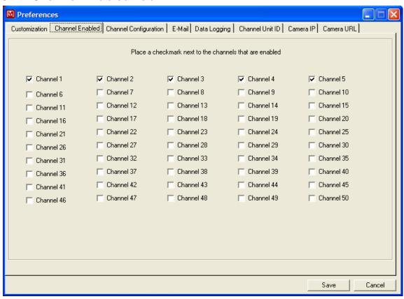
Any channel that is to be used must be marked as enabled first. If a channel is marked enabled and no data is received for a 10-second time interval, the software will indicate that a failure has occurred. Only channels that are enabled will be displayed on the main screen.
