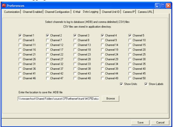
The Data Logging tab allows which active channel will log its data to a file. The location of the database can be specified by clicking on the Browse button. If the units and custom labels are not needed on the main window, un-checking Show Units and Show Labels will remove them.
