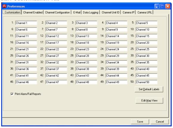
The customization tab allows the channel label to be set and provides access for editing the map view. Printing the alarm and fail reports can be enabled or disabled. Custom labels can be up to 11 characters. Clicking the Default Labels button will automatically reset all channel labels to numerical order: Channel 1:, Channel 2:, Channel 3:, etc.. For more information about the map editor, refer to section 3.4
