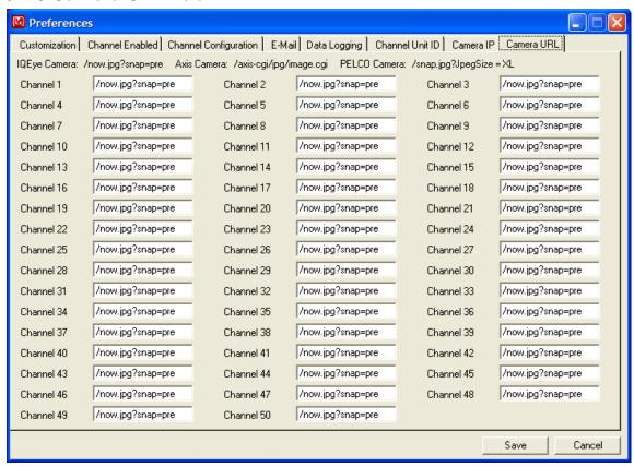
The Camera URL tab sets the URL that is used to get a static image from the camera. Consult your Ethernet camera's documentation for the correct setting. If the URL address is blank, that channel will not capture any images.
