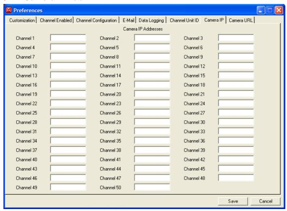
The Camera IP tab sets the IP address for any network cameras that may be installed. If the IP address is blank, that channel will not capture any images. It is possible to assign one camera for multiple channels.
