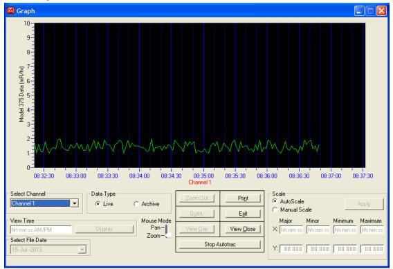
The Graph view displays the readings from the Model 375 as a graph with options to view live or previously saved data (archive mode).
