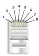
Looking at the connector with the pins at the top facing you, pin 1 is on the left. Pin 8 is on the right.
