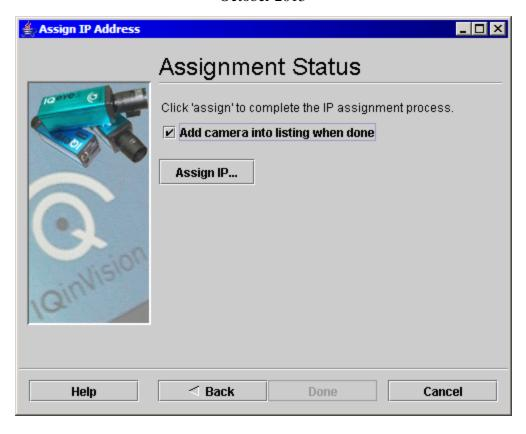
26. Click the Done button. The camera should be added to the VisiCon Main window. Record the IP address on the configuration sheet in Section 5.
