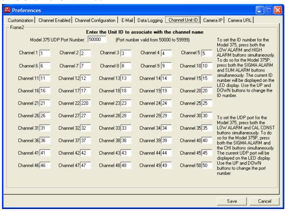
The Channel Unit ID tab associates a specific Model 375 with a specified channel based on the Model 375's three-digit ID number. The UDP port number must be set to the correct value that matches those that all connected Model 375s are using. See Section 2.4 for more information.
