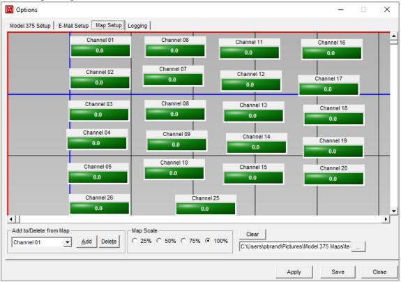
From this screen it's possible to load in a custom map file to be used as a background on the main screen. Once a map is loaded, channels can be added and deleted on the map. Channels can be dragged around to any location on the map.
