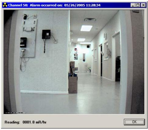
When a high alarm occurs, the image will be displayed in a resizable window along with the date, channel caption, and reading. The images are saved in the images folder under the installation path. The images are named using the following format:
