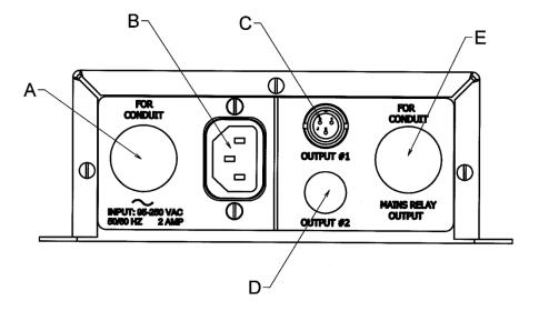
Figure 2. Mains Relay Box Front Panel.
