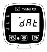
Figure 6.5: Fault - Date Reset.
