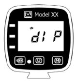
Figure 7.3: Setup - DIP switch protection enabled.
