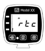
Figure 7.9: Setup Group - Real Time Clock.
