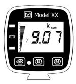
Figure 5.1: Alert example in rate mode.
