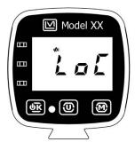
Figure 6.1: Fault - Loss of Counts.
