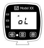
Figure 6.3: Fault - Overload.
