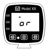
Figure 6.2: Fault - Over Range.
