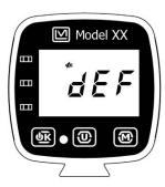
Figure 6.6: Fault - Defaults Loaded.
