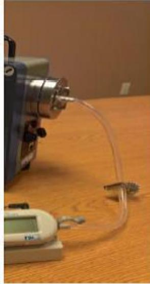
**NOTE:** Ensure that the variable flow restriction does not completely cut off the airflow to the pump. The pump is not designed to pull a high vacuum, and flow rates can damage the pump diaphragm. Do not allow the pump to run below 5 LPM for 7 LPM pumps (or more 4 LPM for 6 LPM pumps) for more than a few minutes.
