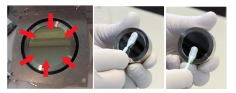
Repeat the cleaning treatment with fresh swabs, as needed, to eliminate traces of contamination. Blow dry with dry air, Ar or N<sub>2</sub> gas, across the detector surface. If possible, put under vacuum for 15 minutes or heat to 50 °C (122 °F) for an hour to remove residual moisture before installing the detector and applying bias.
