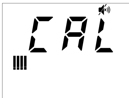
Figure 4.2: Setup Page Selection Display (showing page 4-CAL)
