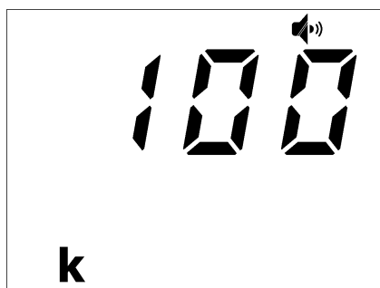
Figure 2.17: COUNT Mode Displaying COUNT Timer of 100k Seconds
