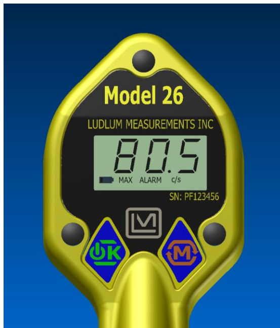
Figure 2: MAX mode operation display with ALARM indicator.
