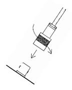
The detector operating voltage (HV) is supplied to the detector via the detector input connector. A mild electric shock may occur if bodily contact is made with the center pin of the input connector. Place the Model 2402 selector switch in the OFF position before connecting or disconnecting the cable or detector.
