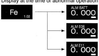
ALM Batt: RED LED lamp flashes. Replace the used battery with new one.
