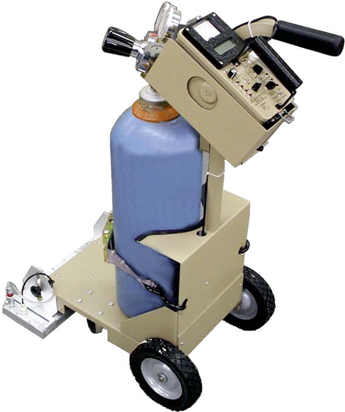
Model 239-1F Floor Monitor shown with Ludlum Model 2221
