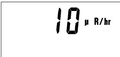
The display will auto-range to the current level (see figure at left). When auto-ranging down, the Model 2241-4 uses multiples of 5. This technique keeps the decimal point from jumping between numbers when viewing values around multiples of 10.
