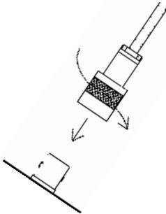
Using the cable provided, connect the Model 42-31H detector to the Model 2241-4; firmly pushing the connectors together while twisting clockwise until the connector latches (a quarter turn) as illustrated in the diagram to the left.
