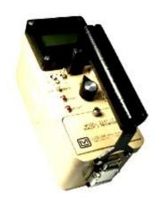
he Model 2241-2i and 2241-2i/2 are portable microprocessor-based digital Scaler/ Ratemeter instruments designed for use with scintillation, Geiger-Mueller (GM), and proportional type detectors to measure ionizing radiation. Data is presented on a four-digit (six digits in the scaler mode) Liquid Crystal Display (LCD) with a moving decimal point. A three-position switch labeled OFF/RATEMETER/SCALER selects the desired operating mode for the instrument.
