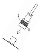
Connect a detector to the survey meter by using the cable provided; firmly pushing the connectors together while twisting clockwise until the connector latches (one-quarter turn). The diagram to the left illustrates how this is done. Next, place the detector selector (INT/EXT) switch in the desired position.
