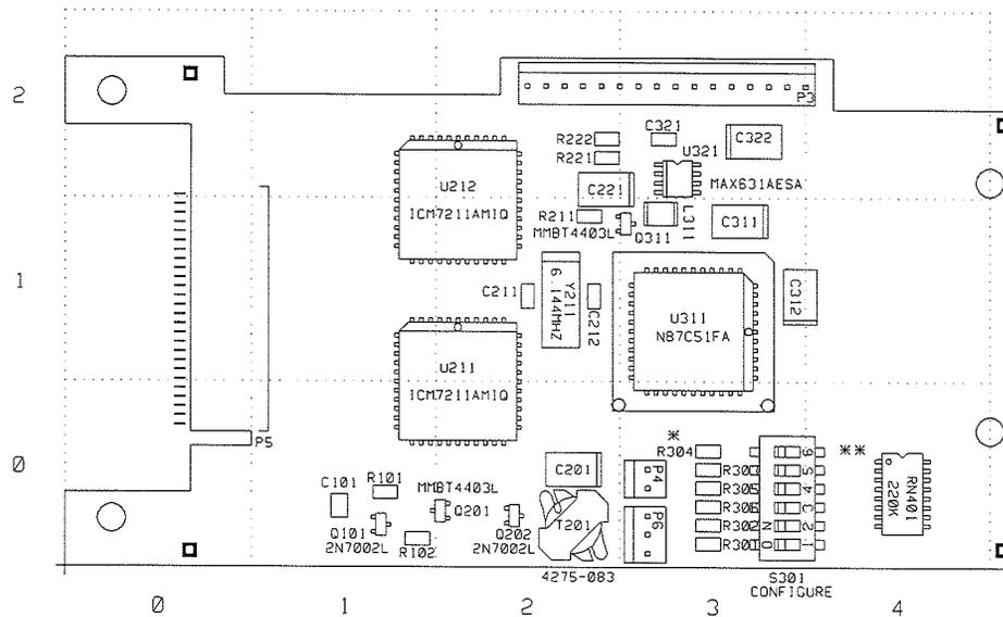
\* REMOVE RESISTOR R304 FOR M2224-3
