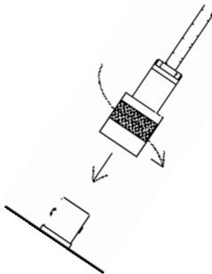
Connect one end of a detector cable to the detector by firmly pushing the connectors together while twisting clockwise one-fourth of a turn. Repeat the process in the same manner with the other end of the cable and the instrument.
