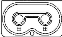
Ensure that the range selector switch is in the "OFF" position. Open the battery lid by pushing down and turning the quarter-turn thumbscrew counterclockwise one-fourth of a turn. Install two "D" size batteries in the compartment.
