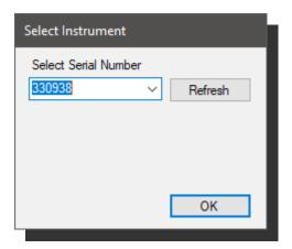
When the application is run, the Select Instrument dialog is displayed. The serial number of the 177-84-2 will be displayed. Select the serial number to change parameters and click OK.
