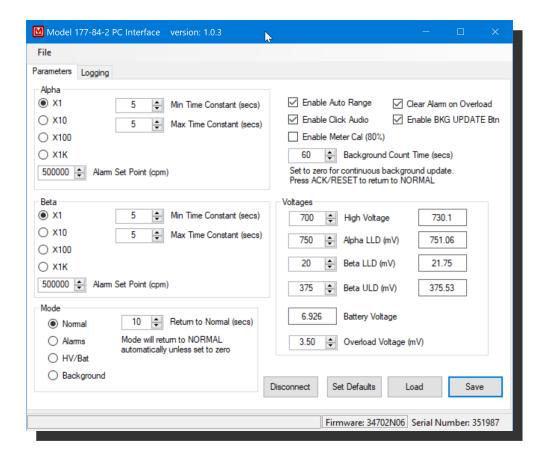
**Alpha Default Range:** Sets the default starting range for the alpha channel. If the count rate exceeds this range, the next higher range will be selected if auto-range is enabled. The default is the X1 range.
