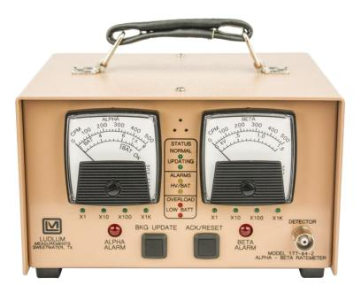
The radiation level is displayed on two analog meters. The Alpha meter dial indicates 0-500 cpm with range multipliers of X1, X10, X100, and X1000. The Beta meter dial indicates 0-500 cpm with range multipliers of X1, X10, X100, and X1000. The meter range may be fixed or auto-ranging, depending on PC Interface software settings. Each channel has its own distinguishable click-per-event audible tone. Beta events are a low pitch and alpha events are a high pitch.
