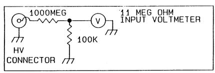
Multiply voltmeter reading by 10,000 for actual high voltage output.
