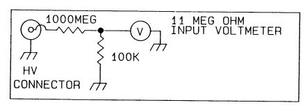
Multiply voltmeter reading by 10,000 for actual high voltage output.
