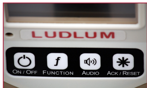
Model 9DP-1 control panel
