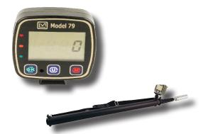
The Model 79/2 has three modes of operation - RATE, MAX, and COUNT. Measurements can be collected in two sets of units (primary and secondary) for RATE and MAX modes in cps, cpm, Sv/h, mrem/hr, and R/hr units. The user can choose by simply pressing the Units button. An internal switch is used to enable or disable the front-panel setup feature to protect desired settings from inadvertent modification. Setup is also available via software from Ludlum Measurements.
