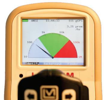
These instruments were the very first ones designed to meet ANSI N42.34 Performance Criteria for Handheld Instruments for the Detection and Identification of Radionuclides. The design was also optimized for portability, user-friendliness, and rugged use out in the field.
