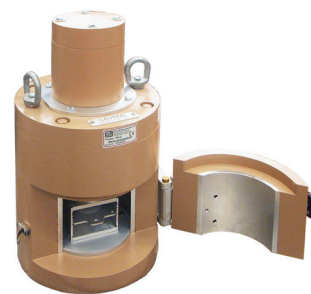
Above: Optionally available Sample Holder for low background sample counting. Model 180-9 Part Number 47-1591
