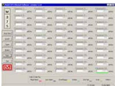
The main window displays reading boxes for all 50 Model 375s along with their status, units, and caption. Clicking on the channel name will display the last image and alarm information that has occurred since the program was running. Holding the mouse over the channel name will display a tool tip with the user-defined comment.
