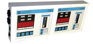
The Model 375-Dual is a dual-channel area monitor controller based on the legacy version of the Model 375. It consists of two Model 375 controllers in one wall-mount chassis, each with its own detector connection. A common application is gamma and neutron monitoring: one controller monitors gamma radiation and the other monitors neutron radiation. This instrument may also be used to monitor radiation in two separate locations when used in conjunction with appropriate external detectors.
