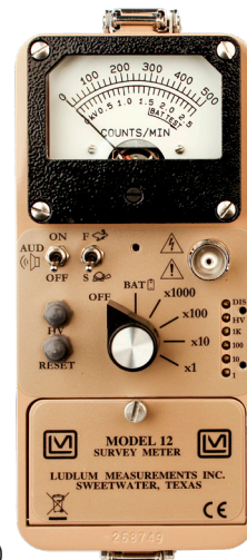
Model 12 face, shown with handle removed for clarity
