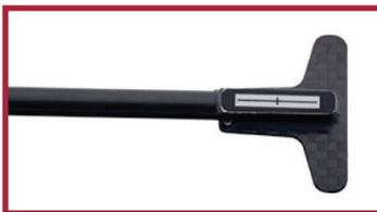
**T20 Dose Detector:** Measures patient entrance dose (skin dose) and maximum dose rate in radiographic and fluoroscopic fields. Its small size eliminates an effect on system output or the X-ray beam. It has a built-in correction filter for different beam energies, thereby producing a flat energy response without the need to compensate. Energy independency, measuring range, and angular dependency fulfill the IEC directive for dose detectors (RQR50-150kV).
