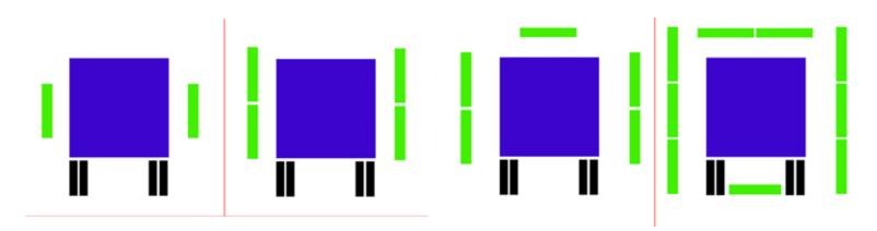
By adding more of the large size detectors, you get greater coverage, enhancing your probability even more. The takeaway principle is easy to grasp; large detectors and more detector coverage results in greater probability of detection.
