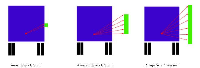
Placing a small sized gamma detector at any point within a gamma radiation field will result in exposure to a relatively small portion of the overall radiation. In real-world metal recycling conditions, a uniform shaped radiation field (sphere) will rarely, if ever, exist, and will, therefore, be highly distorted or directional. A small sized detector will in all probability miss the radiation. As the diagram above depicts, a larger detector has a greater probability of seeing the radiation.
