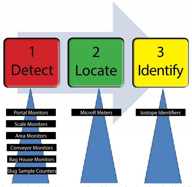
Radiation detection is available in three stages to facilitate all the needs of metal recycling and smelting facilities.
