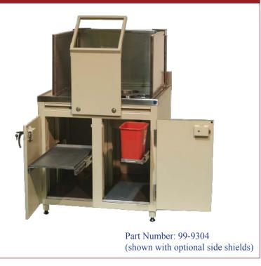
As shown above, three optional side shields are available for the top of the cabinet. The shields, Part Number L-995-037S, are 1.3 cm (0.5 in.) lead covered with stainless steel and fit into "L" brackets with two vertical corner gussets.
