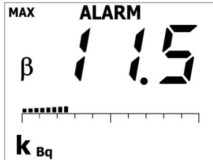
Figure 2.9: MAX Mode Display With ALARM Indication
