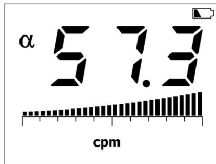
Figure 2.8: RATE Mode Displaying Background Radiation Rate
