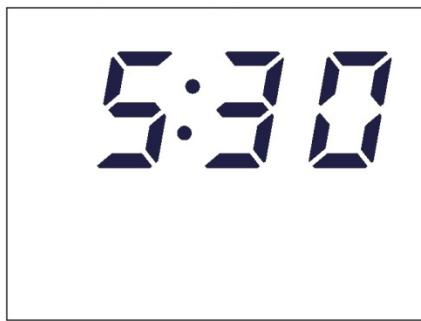
Figure 2.10: COUNT Mode Displaying COUNT Timer of 5 Minutes, 30 Seconds
