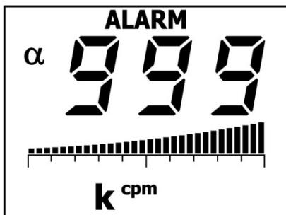
Figure 2.6: Detector Over Range-Alpha (Display Will Flash)
