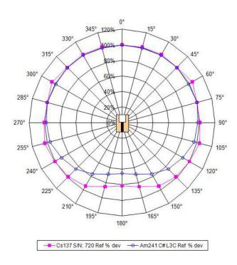
**Magnetic Field Testing:** per ANSI 42-17A-2003,  $\leq$  15% change in readings when placed into a magnetic field 800 A/m, rotated on three axes
