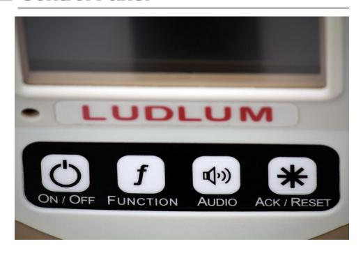
The instrument is equipped with a four-button control pad, as shown above. All controls for the instrument are performed via these four control buttons. Each labeled button has set operation(s) it performs.
