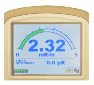
The Ludlum Model 9DP-1 is equipped with a color LCD that improves the user's understanding of the instrument reading, functions, and operating status, as compared to other typical display technologies. The LCD utilizes a bit-mapped layout to afford an optimized arrangement of all of the data available.
