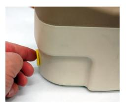
An operational test is performed by placing a radioactive check source against the detector to induce an upscale reading. Ludlum recommends a 10  $\mu$ Ci <sup>137</sup>Cs check source for this purpose. This is an exempt quantity in the USA so no license is required to purchase and receive this source. You can purchase it from Ludlum by ordering Part Number 01-5231. Several other countries only permit 0.25  $\mu$ Ci <sup>137</sup>Cs as an exempt status, so check your local regulations.
