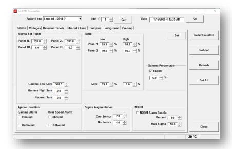
The Alarms tab is used to set the radiation alarm set points and if a gamma or over speed alarm is ignored for a particular direction.
