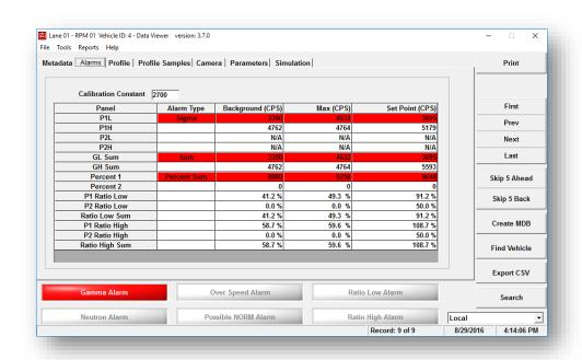
The Alarm tab displays the status for each detector panel and sum channel for the current record. The alarm type, background reading, max reading during the occupancy, and set point (if enabled) are shown. Any detector panel or sum channel that alarmed will be highlighted in red.
