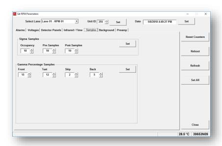
**Occupancy Samples:** Sets the number of 100-millisecond samples that must occur before checking for an alarm. The RPM should be rebooted after changing this parameter.
