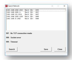
Click the Search button to begin searching for RPMs. When all available RPMs have been found, click the Save button. As each RPM is found, the Supervisor software retrieves its unit ID and displays it next to the IP Address. The Supervisor software displays several codes when retrieving the unit ID if a problem occurs. They are:
