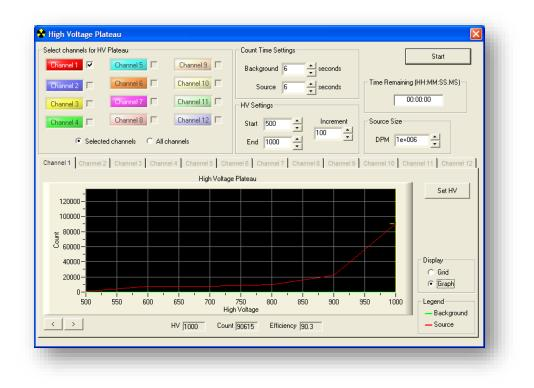
Once the plateau is complete, clicking on the "Set HV" button will set the high voltage and efficiency for the channel. Select the appropriate high voltage and efficiency by highlighting the row on the grid or by selecting a point on the graph with the cursor. On the graph view, the cursor can be moved by dragging it around the plot with the mouse or by using the "Cursor Left" and "Cursor Right" buttons, which are located at the bottom left corner of the graph.
