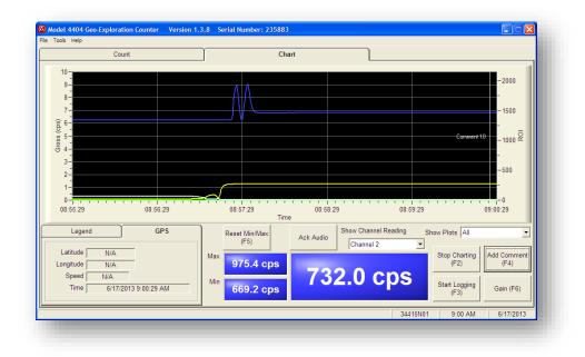
The current GPS coordinates are displayed along with the speed and date/time reported by the GPS receiver. A read out displays the selected channel's current count along with a minimum and maximum value large
