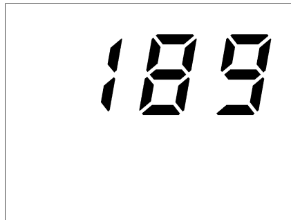
Figure 2.4: Startup Display Showing 189 Stored Data Records
