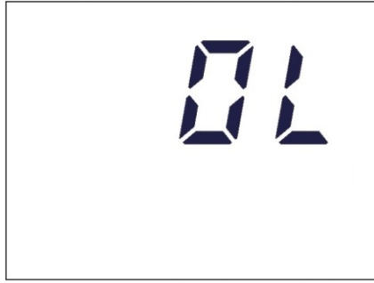
Figure 2.7: Detector Overload Alarm (Display Will Flash)
