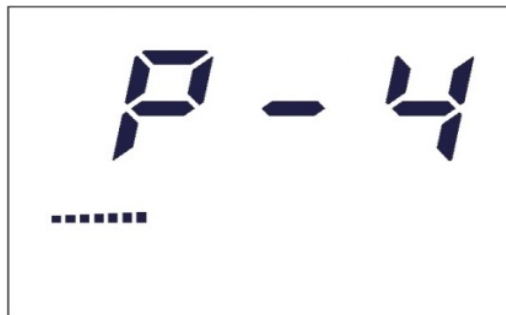
Figure 4.1: Setup Page Selection Display (showing page 4-CAL)
