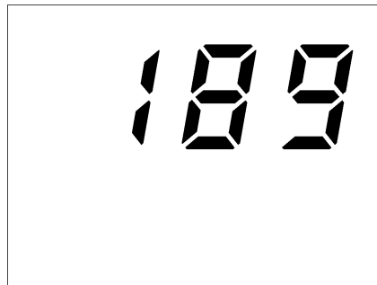
Figure 2.4: Startup Display Showing 189 Stored Data Records
