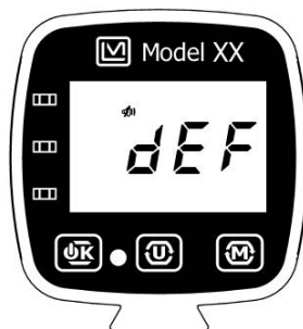
Figure 6.6: Fault - Defaults Loaded.
