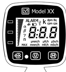
Figure 4.1: Startup display with all LCD segments shown.
