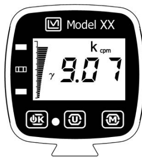
Figure 5.1: Alert example in rate mode.
