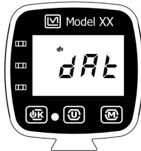
Figure 6.5: Fault - Date Reset.
