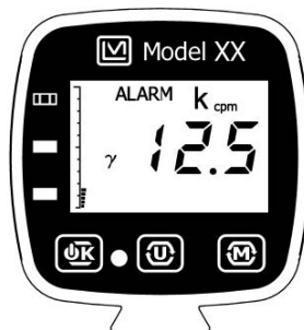
Figure 5.2: Alarm example in rate mode.
