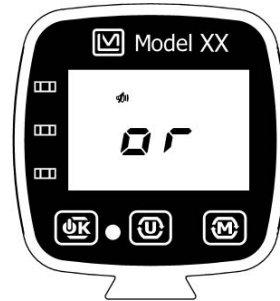
Figure 6.2: Fault - Over Range.
