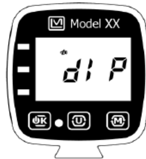
Figure 7.3: Setup - DIP switch protection enabled.
