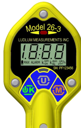
Figure 1: Startup display for Model 26-3, with all LCD segments shown.
