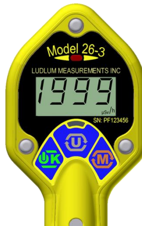
Figure 4: Detector Over Range (shown for \mu\text{Sv/h} ); will also flash.
