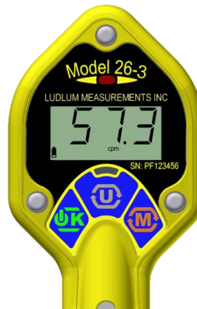
Figure 5: RATE mode display showing typical background radiation rate and the low-battery icon.
