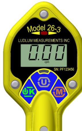
Figure 3: Detector Failure display (shown for cpm); will also flash.
