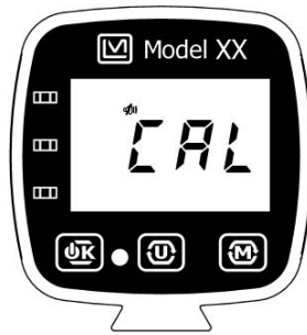
Figure 6.4: Fault - Calibration Expired.
