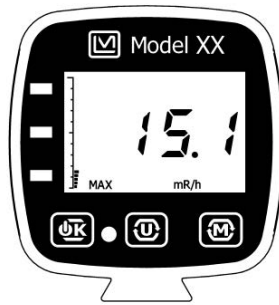
Figure 5.4: MAX mode display.
