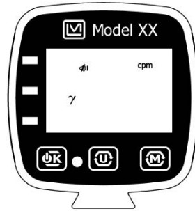
Figure 5.5: Entering COUNT mode from another mode or changing units within COUNT mode.
