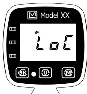
Figure 6.1: Fault - Loss of Counts.
