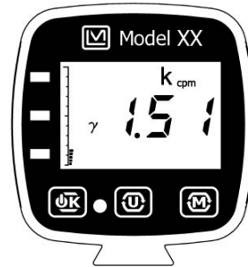
Figure 5.3: RATE mode display.
