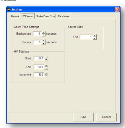
The plateau settings determine the default values used when running a plateau. These values can also be changed directly on the HV Plateau screen.
