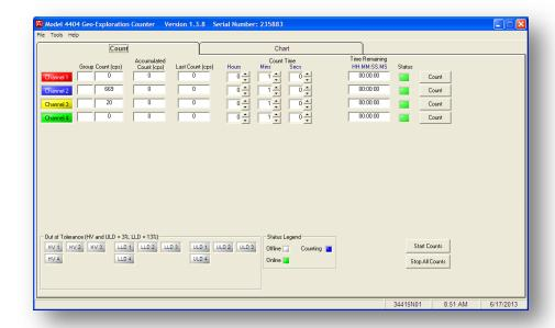
The main screen displays the following information: current one-second count, accumulated count, last count, status, and out-of-tolerance.
