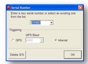
After connecting a different Model 4404-16, select Change Serial Number from the Tools menu and select the correct serial number from the drop-down list. If this is a new counter, enter in the serial number.
