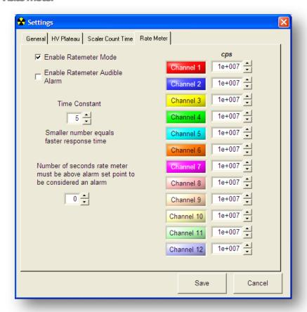
The rate meter settings determine if the rate meter is enabled and what the time constant will be when enabled. This setting affects the count values on the chart and the values saved to the data file. When disabled, the count is the raw one second count. The higher the time constant the slower the response time will be.
