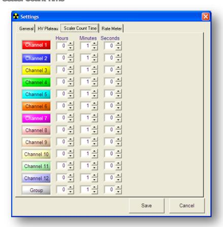
The scaler count time settings determine the default values used for the count times. These values can also be changed directly on the main screen.
