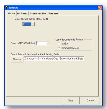
**COM Port:** The RS-232 serial port is used to communicate with the counter. This list box displays all available communication ports on the computer. If a USB-to-serial adapter is used, consult the documentation that came with it for instructions on installing any drivers and configuring the port.
