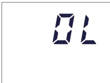
Figure 2.6: Detector Overload Alarm (Display Will Flash)
