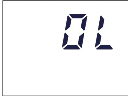
Figure 2.7: Detector Overload Alarm (Display Will Flash)
