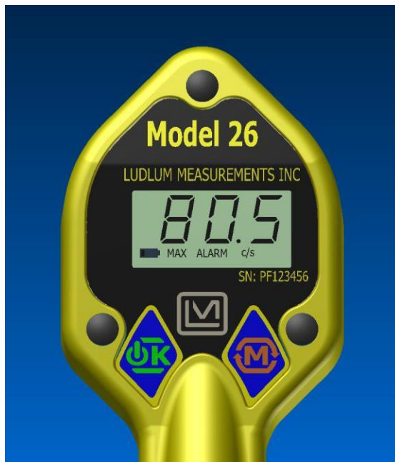
Figure 2: MAX mode operation display with ALARM indicator.
