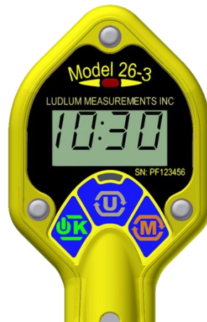
Figure 7: COUNT mode operation showing COUNT Timer of 10 minutes, 30 seconds.
