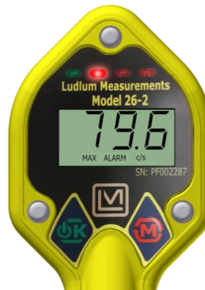
Figure 2: MAX mode operation display with ALARM indicators for Lowest Alarm Level. A single red LED will be flashing.
