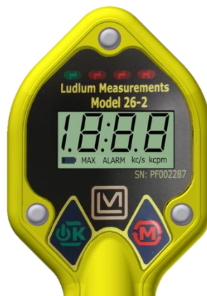
Figure 1: Startup display for Model 26-2, with all LCD segments shown.
