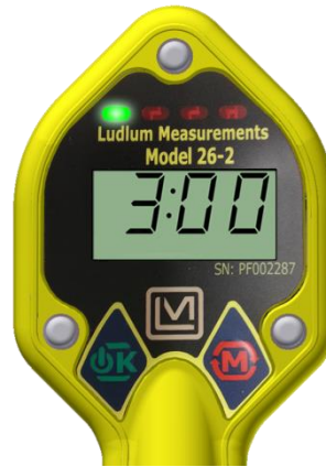
Figure 3: TIMED FRISK mode operation showing Frisk Timer of 3 minutes. Green LED will be steady ON.
