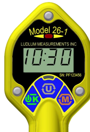
Figure 7: COUNT mode operation showing COUNT Timer of 10 minutes, 30 seconds.
