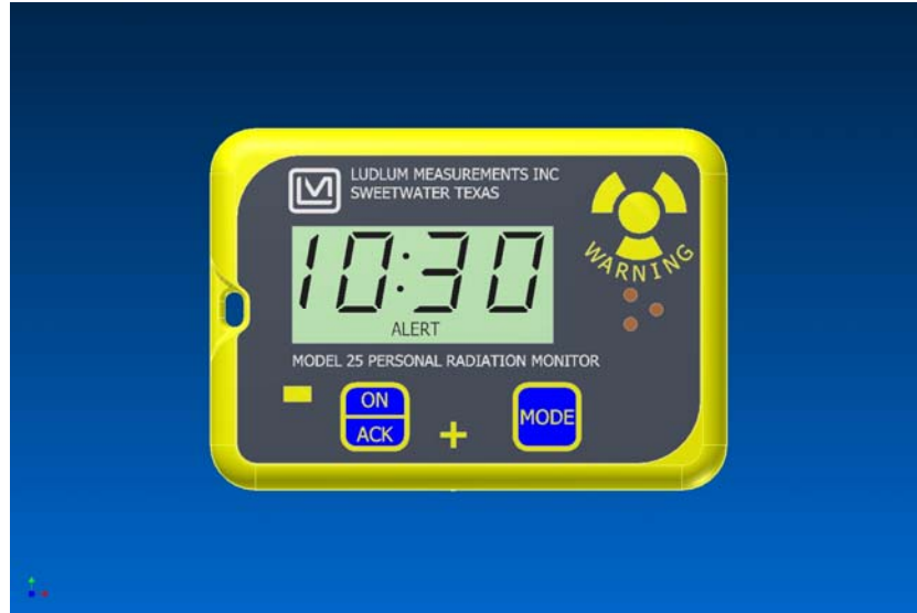
Figure 3: Time Remaining Screen with ALERT indication
